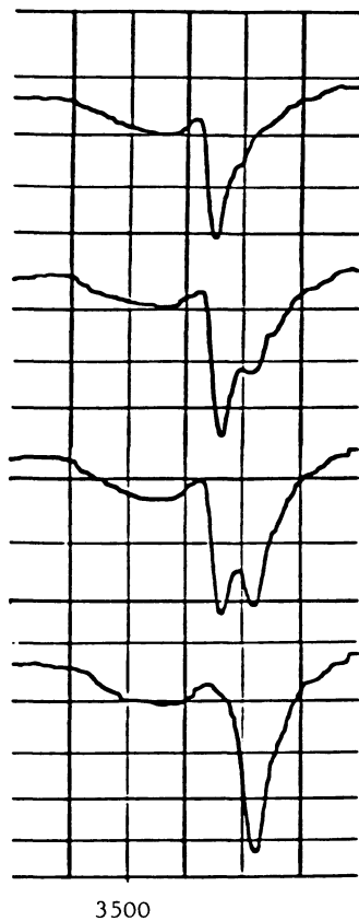
Figure 5. IR Spectra of N-H Stretch Region. All spectra are Time Composites Taken on Samples of Benzanilide Exposed to 6000 ppm Bromine at pH 3.0.
